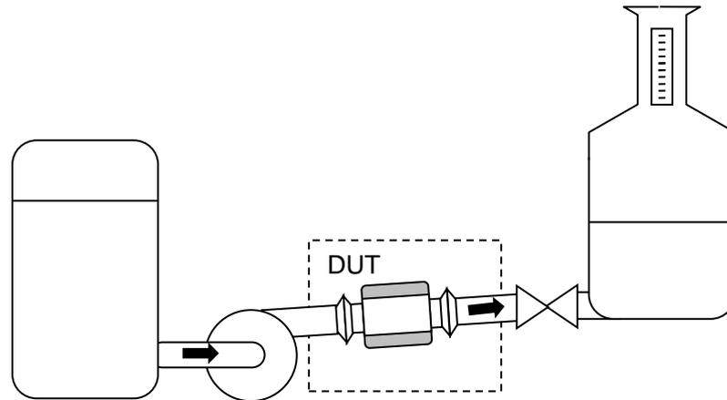
The illustrated arrangement pumps water from a tank through the volume meter to be verified, through the counter-pressure valve, and into a tank.
