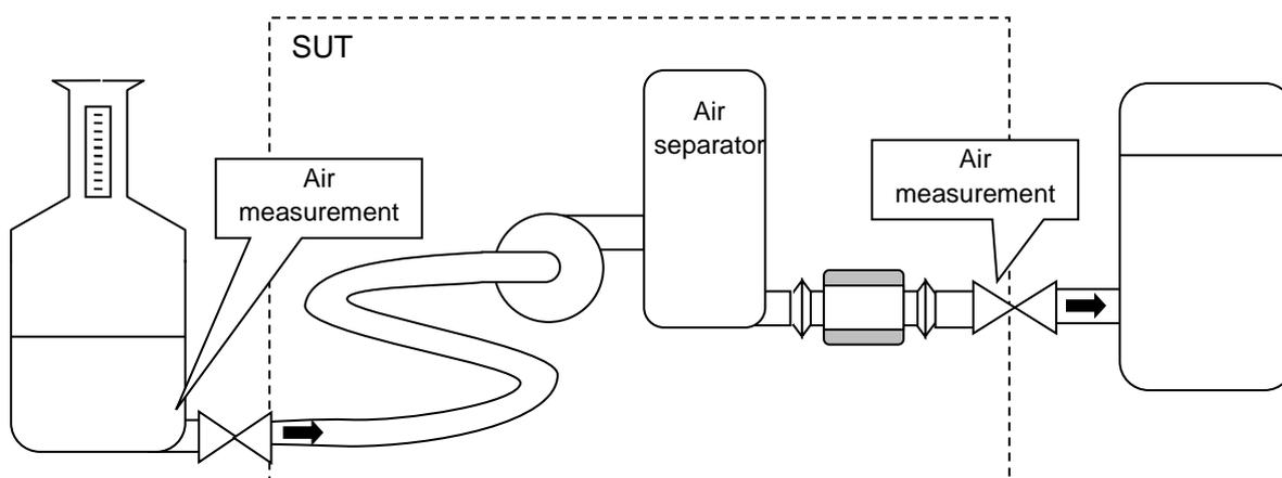
The reference tank is filled with water to a known volume including the valve. After that, a hose is connected to the weighing tank. The valve is opened, the tank is emptied, and finally the hose is dismantled and rolled up, or placed in accordance with the enclosed instruction.
