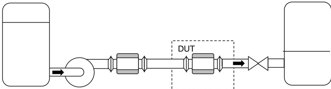
The illustrated arrangement pumps water from a tank through a verified volume meter, followed by the flow transmitter that requires verification (DUT = Device Under Test), through the counter-pressure valve and into a tank.
