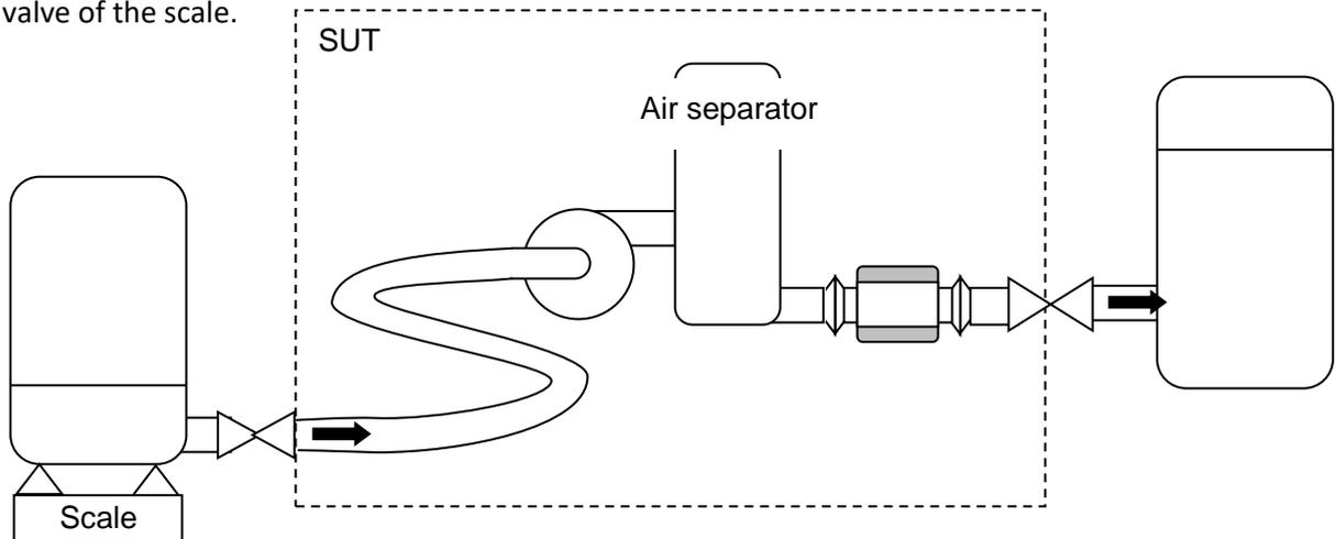
A tank on a scale is here used with a bottom valve as reference, corresponding a farm tank.
