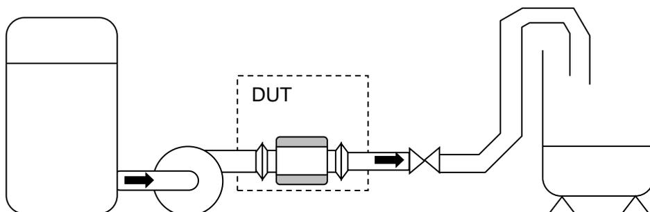
In the illustrated model the liquid is pumped through the volume meter via a constant pressure valve into a tank on a calibrated scale. The weight indication must be compensated for the water's specific gravity, the temperature, etc. See section 2.
