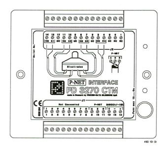
The unit provides high resolution measurements of a value related to conductivity. The continuous fully integrating non sampling principle offers high noise immunity. The influence of periodic disturbances can be damped with the adjustable averaging function.
